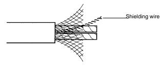
3. Remove the exposed weaving and the aluminum tape from the signal and power lines. Strip the covering from the signal and power lines to the proper length for the crimp terminals. Twist together the wires of each of the signal and power lines.
